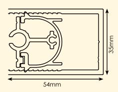
This track is designed to be recessed into wall cavities or columns
