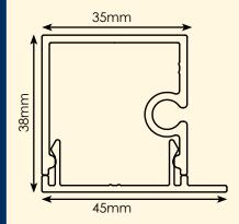
The standard track is for face fit and reveal installations
