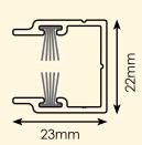
The Standard Track is designed for maximum mesh retention in most applications whilst the Small Track has been introduced for internal shading where wind is not a factor
